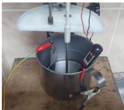
Fig. 1. Experimental setup used for the plasma electrolytic oxidation (PEO) treatment of the AZ31 magnesium alloy.
