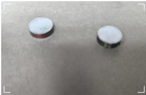
Fig. 1. Treated Ti 25 Ta 25 Nb 3 Sn disc, 10 mm × 4 mm.
