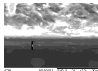
Fig. 3. SEM analysis of a HIPS showing the film formation deposited on the HIPS.
