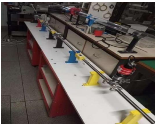
Fig. 1. Image of the high vacuum tubular system constructed with different experimental pressure measurement positions.
