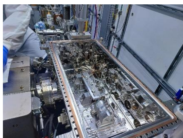
Figure 3: Mirror system working in UHV regime and partial pressure of oxygen to reduce the carbon contamination.
