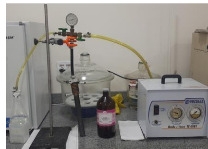
Fig. 3. Vacuum application for density testing.
