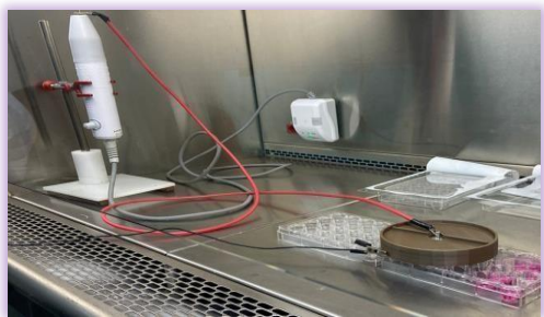
Fig. 1. Exposure of microbial species and Vero cells in a 24-well plate to the plasma generated by the equipment.
