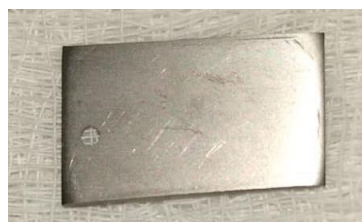
Fig. 2. Nb sample sanded with 1000 grit sandpaper.
