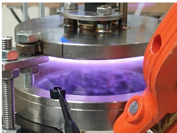
Fig. 1. CNTs samples mixed with MA being treated in glow discharge provided by ABiPPS in CCP reactor.
