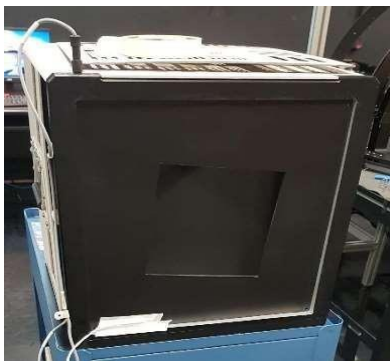
Fig. 1. Set up used for the camera Spatial resolution measurement.
