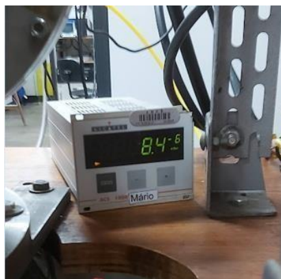
Fig. 7. The new system base pressure after 1 hour of pumping.
