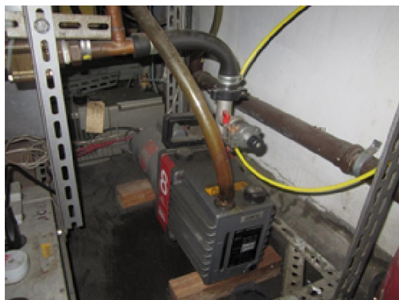
Fig. 1. Mechanical pump connected to the 3IPLAP vacuum chamber and to the diffusion pump.
