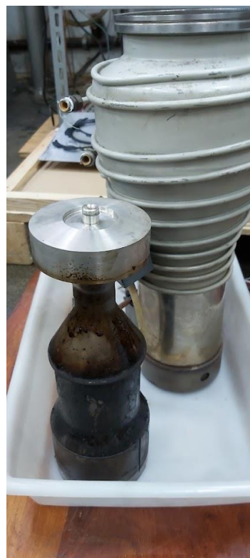
Fig. 4. The diffusion pump was dismantled. The internal parts were covered with a thick layer of burnt oil. The removal of the deposited layer involved mechanical and chemical cleaning.
