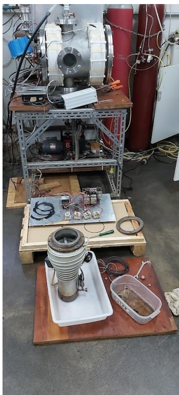
Fig. 3. Diffusion pump removed from the vacuum system.
