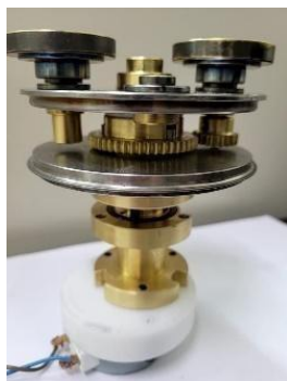
Fig. 1. Planetary rotating sample holder and low-cost rotational mechanical through-hole.
