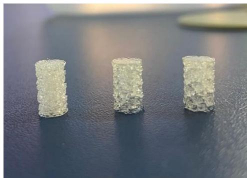
Fig. 1. Porous polymeric samples, as tested.
