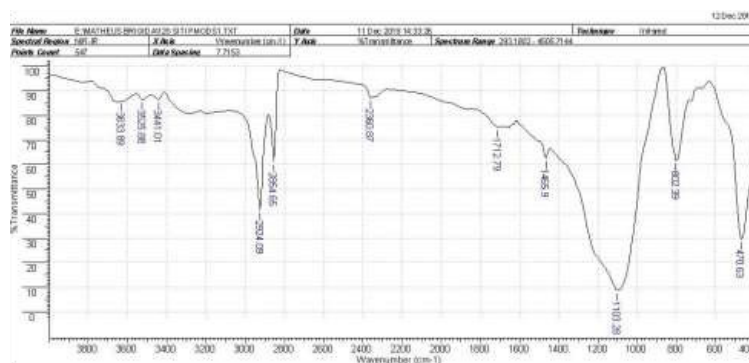
Figure 1: Fourier transform infrared spectrum for solid phase extraction sorbent prepared at 120 °C for 12 h.
