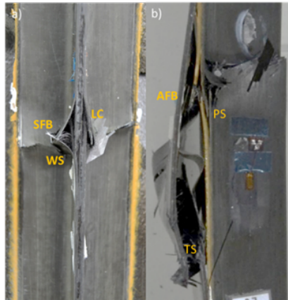
Figure 1: Failure modes observed at CB panel after catastrophic failure.
