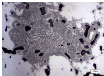
Fig. 1. Microstructure after sintering for 1h.
