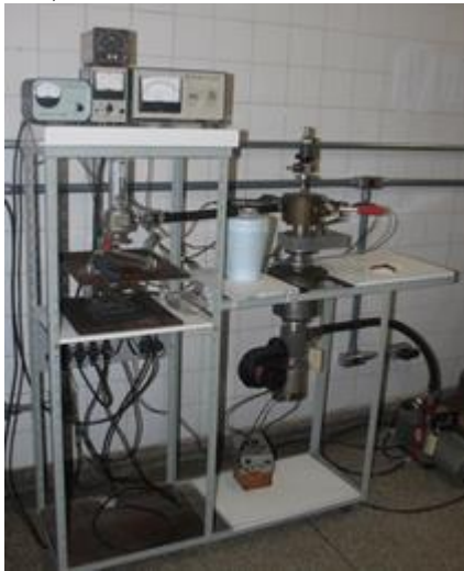
Fig. 1. Overview of vacuum chamber, pressure gauges, both mechanical and diffusion pump and nitrogen trap.
