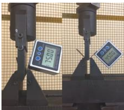
Fig. 1. U bending test for predetermined angles of 30° and 90° respectively. Predetermined angles that appear in the image refer to the x axis.
