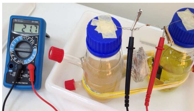
Fig. 2. Set-up of H-shaped microbial fuel cells, constructed to evaluate the performance of a carbon fiber electrode.
