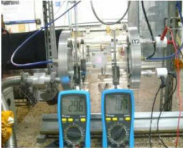
Fig. 1 Discharge chamber and electrical measurements equipment's [7].
