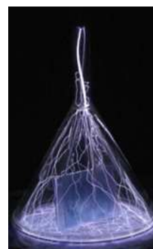
Fig. 2. Photo of a plasma jet with vertical sample
