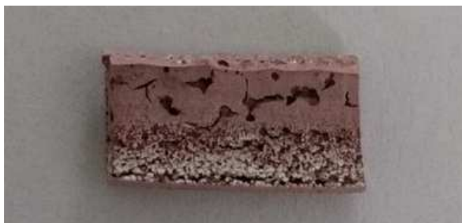
Figure 2. Side cut of sample 1, showing non-homogenization
