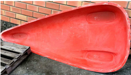
Fig. 4. Mold after spray up process, bottom view.
