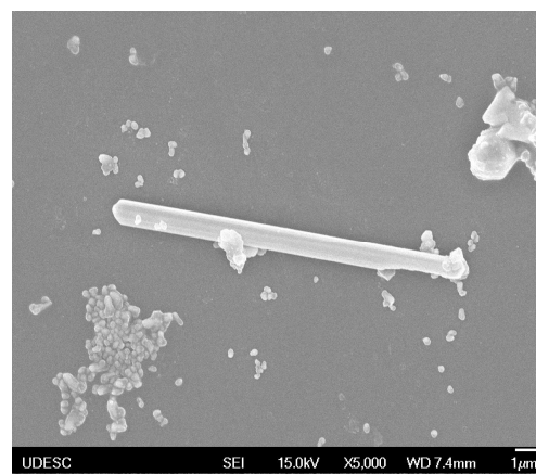
Fig. 2. SEM image showing a Ag/PPy columnar crystal, after 72h of reaction.
