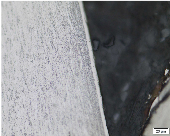
Fig. 3. A576-2h sample compound layer.
