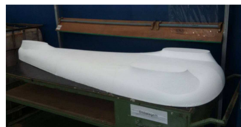
Fig. 3. Plug in polyurethane after machining.
