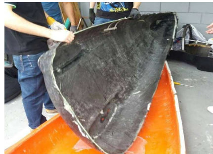
Fig. 5. Composite unibody demolded.
