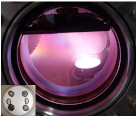
Fig. 1. In the corner of this image, the arrangement of Bario / Strontium Titanate tablets glued to the silver target is shown. In the larger image, the RF discharge with argon gas. There is a great luminosity throughout the deposition chamber.
