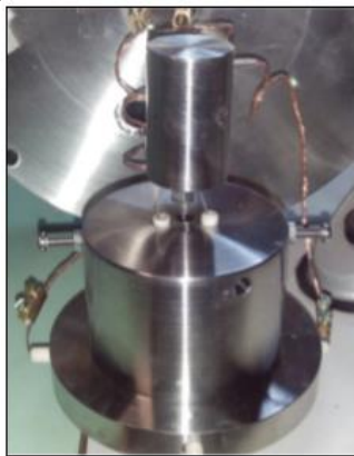
Fig. 1. Vacuum electric oven mechanical assembly.
