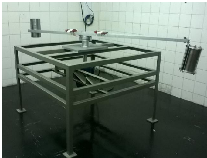
Fig. 1. Centrifuge (with furnace at the right side) of LAS/INPE.
