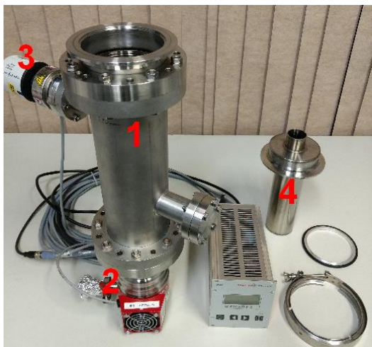
Fig. 1. The experimental setup used during the proof of concept tests. The chamber 1 has a volume similar (5 liters) to what we expect for the fast entry. The system was pumped by a Pfeiffer HiPace 80 turbo molecular pump (2) and the pressure measured with a Pfeiffer PKR-261 full range gauge (3). The cryogenic pumping was obtained filling a 300 ml LN 2 trap (4).
