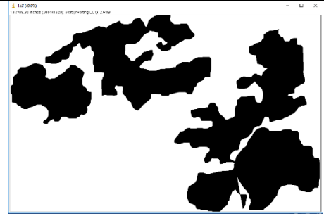
Fig. 4. AA7050-T7451 alloy optical microscopy: coarse grains distribution.
