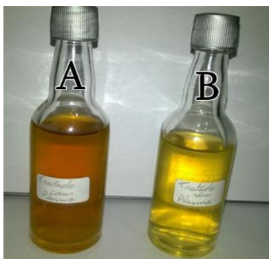
Fig. 1. Image of solubilized lignin extracted from corn, A being treated with plasma and B with control treatment.
