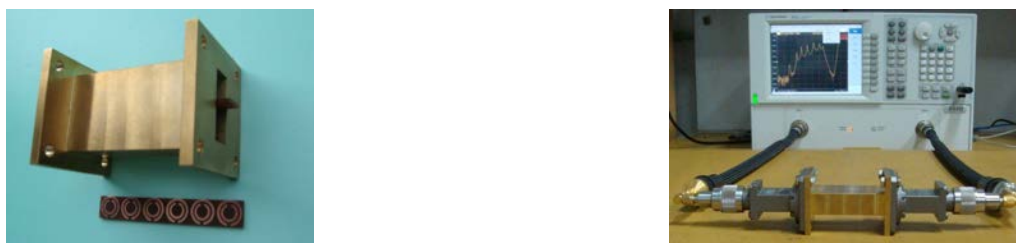
Fig. 1. (a) WR90 waveguide loaded with six SRRs. (b) Set-up to measure scattering parameters in the X-band waveguide loaded with the SRR array using waveguide coaxial adapters.
