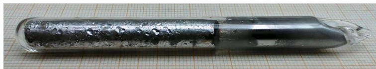
Fig. 2. PbSn eutectic alloy sealed in a quartz ampoule.
