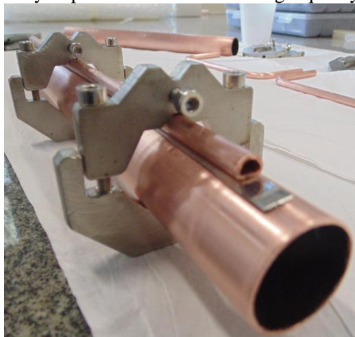
Fig. 2 Detail of the assembly of the vacuum chamber, refrigeration tube and metal addition with the special device before brazing procedure.
