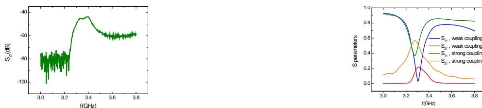
Fig. 2 (a) The transmission band for the waveguide loaded with a periodic array of six SRRs measured with coaxial-waveguide adapters. (b) Magnitudes of reflection ( S_{11} ) and transmission ( S_{21} ) scattering parameters. Measurements were made by using magnetic probes.
